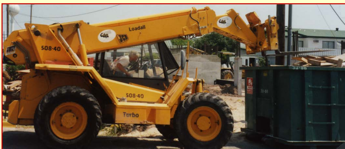
Fig. E8.7 A Loadall unit equipped with a pair of forks for lifting pallets.
