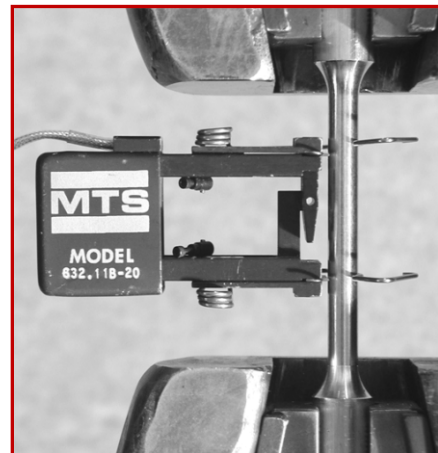
Fig. 3.19 A tension specimen with an extensometer for measuring the deformation \delta .
