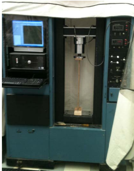
Fig. LRT 2 The Instron machine used to apply an axial tensile force to the tensile specimens.
