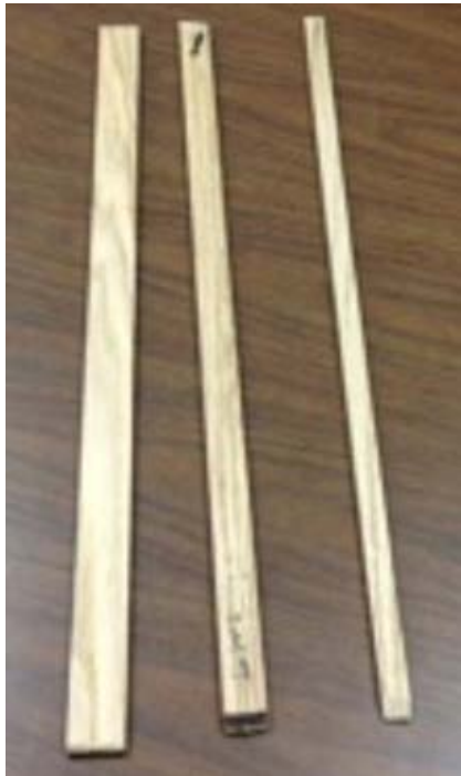
Fig. LR3. Column specimens fabricated from oak with longitudinal grain orientation.
