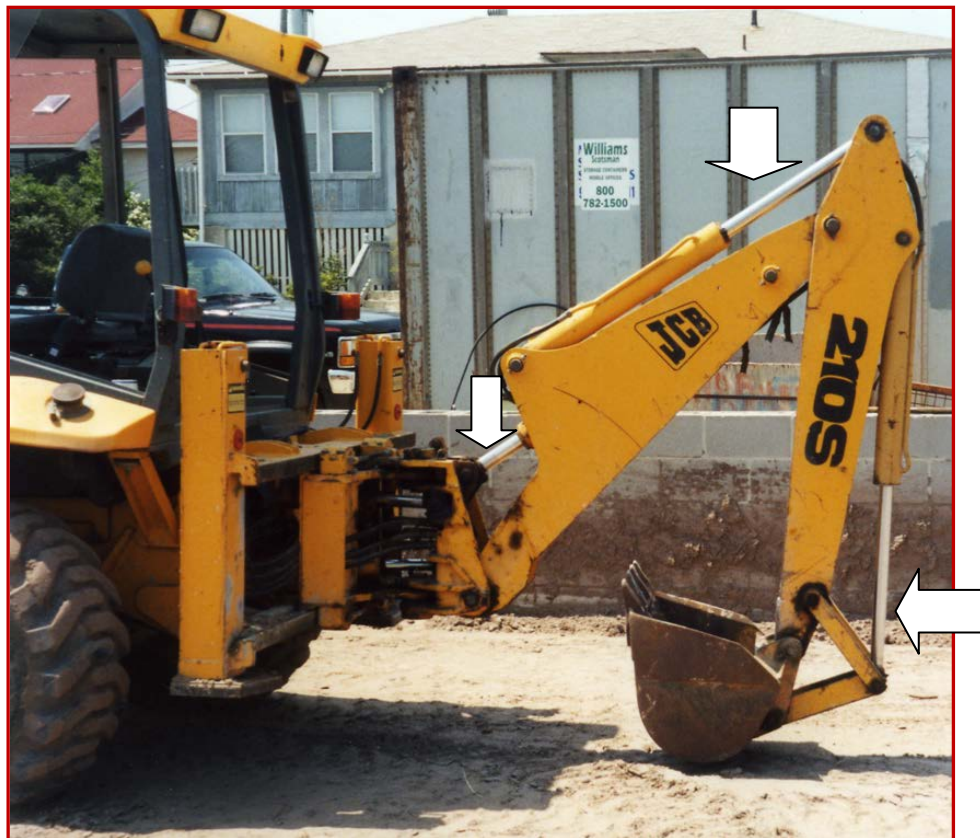
Fig. 8.3 Hydraulic cylinders actuate the arms and bucket on a backhoe.
