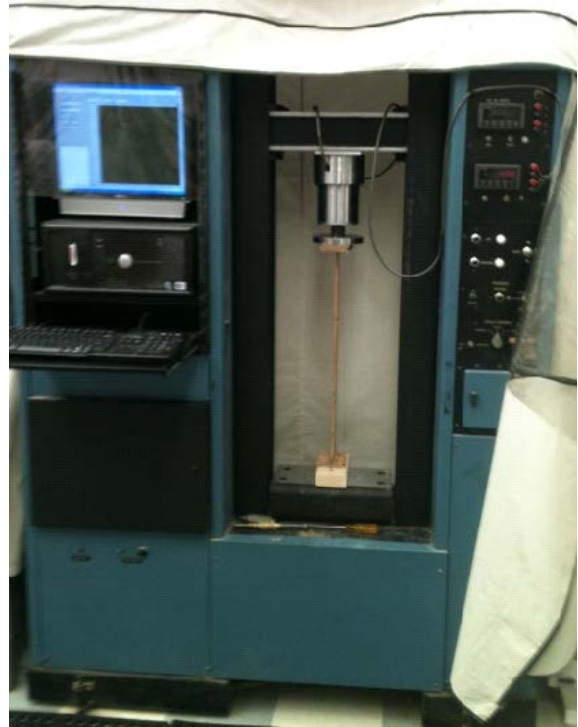
Fig. LR2 The Instron Machine with wooden column ready for the test.
