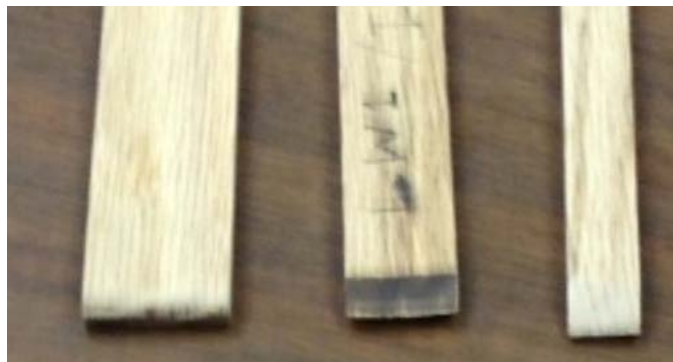
Fig. LR4 Specimen ends were rounded or sharpened to simulate the pinned end condition.
