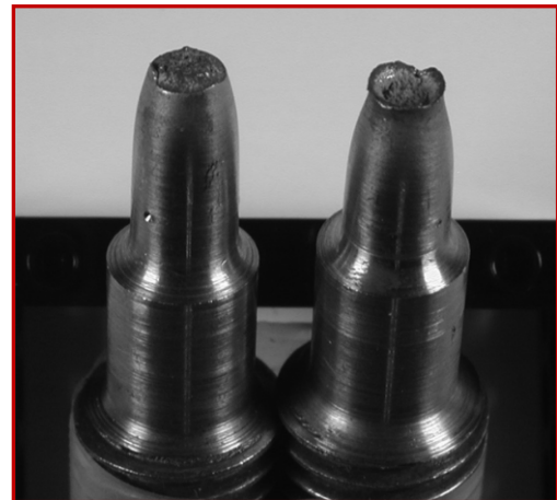
Fig. 3.23 Ductile failure of a tensile specimen. Note the cup and cone fracture region
