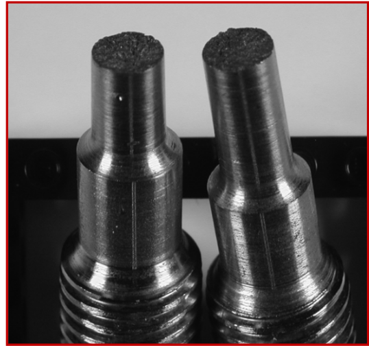
Fig. 3.21 Failure of a brittle material occurs suddenly with little plastic deformation.
